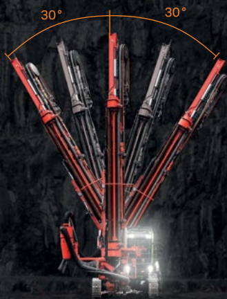
FEED SWING DRILLING ANGLES
